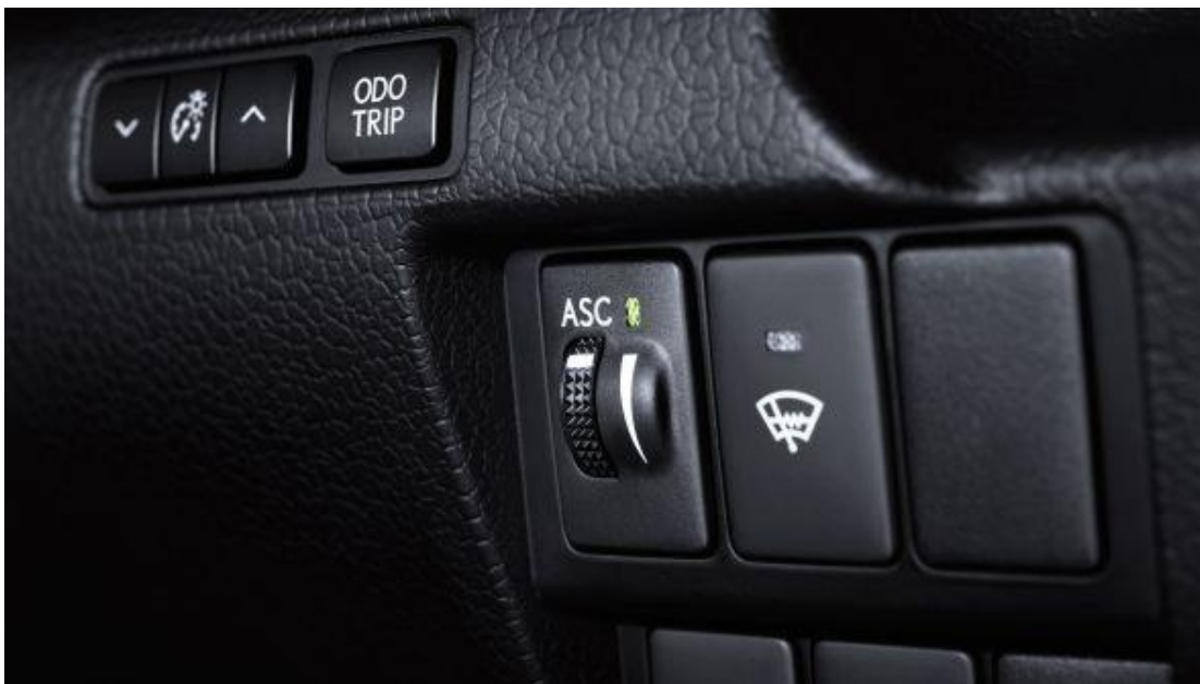
Figure 3. Some Lexus models include Active Sound Control (ASC), a volume-adjustable "new technology that compliments [sic] the sound of the engine with an audio feed through a dedicated loudspeaker hidden behind the dashboard." 26 The combination of design theater with this explicit driver-facing control mechanism—a strange confluence
